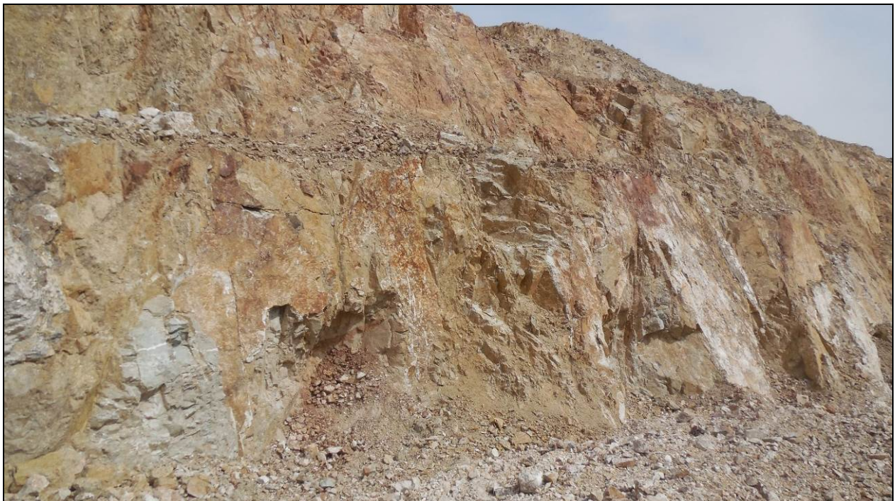
Figure 16-5: Existing Phase I pit wall showing footwall trace of Moss Vein
