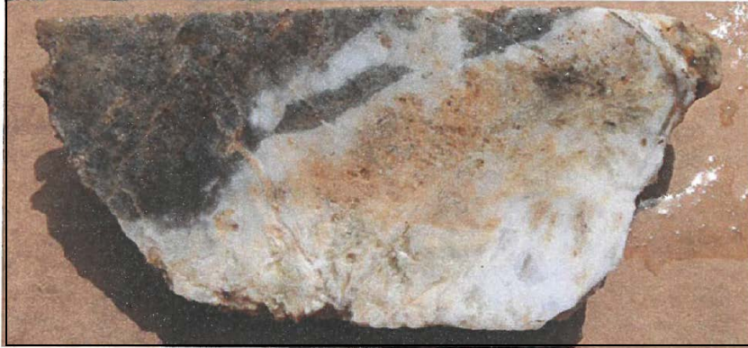
Figure 7-5: An Example Quartz Vein Material with Bladed Texture from Calcite Replacement and Showing Limonite Staining (oxidation) along a Joint Plane (drillhole AR-69C, 80.77 m)
